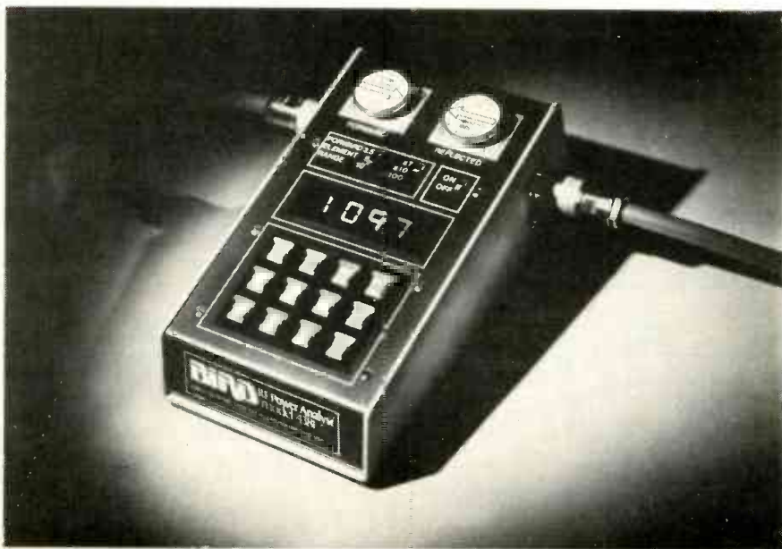
A MODERN INSTRUMENT FOR MODERN TRANSMITTERS. The Bird 4381 RF Power Analyst measures forward and reflected power for CW, AM, FM, and SSB (peak envelope power), automatically calculated VSWR, %-AM modulation, and return loss. It keeps track of maximum/minimum values, and identifies a rise or fall in measured values. Though jam-packed with features, just about all are a "must" for the modern service technician.
