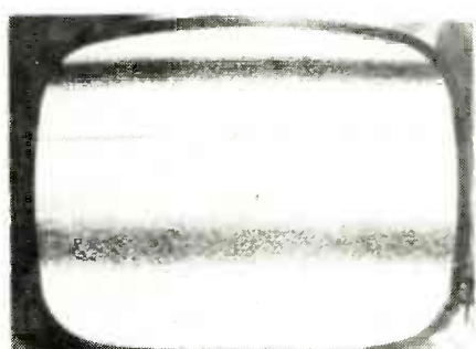
FIG. 1—DOUBLE LINES of hash indicate 120-Hz rate of AC power-line noise.
