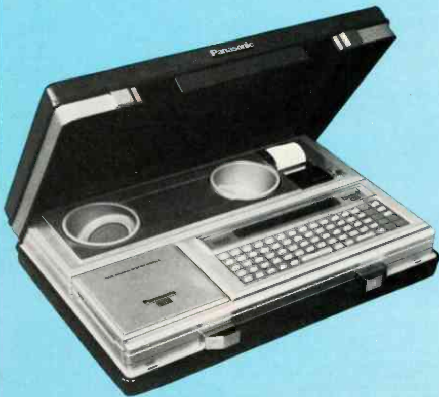
PANASONIC HAND-HELD COMPUTER RL-H1000, shown here in a briefcase combination with cassette interface, acoustic coupler/telephone modem, and mini-printer.
