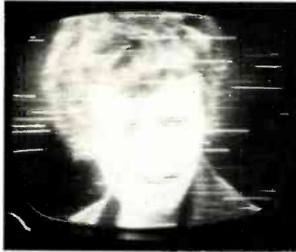
FIG. 6—IGNITION NOISE from vehicles without suppressors may cause this.
